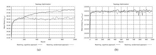
Figure 2. (a) Fitness function that shows the mean number of retrieved items per node. The fitness of the randomized algorithm is represented as the dashed line, our approach as the solid line. (b) Mean energy usage per node of the randomized algorithm (dashed) and our approach (solid).
